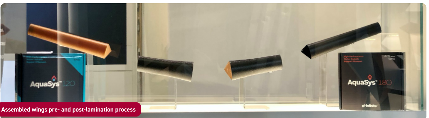
Carbon fiber-laminated wing after core removal
