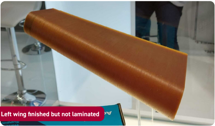
Pre-assembled wings printed with AquaSys 180 before Carbon Fiber Reinforced Polymer (CFRP) lamination
