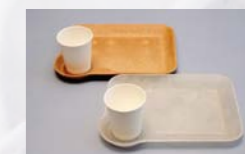
Pullulan/Biodegradable Plastic (Top: combined with cypress; Bottom: unmixed pullulan)
